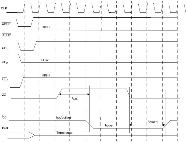
Device must be deselected when entering ZZ mode. See Cycle Descriptions Table for all possible signal conditions to deselect the device. I/Os are in three-state when exiting ZZ sleep mode.
